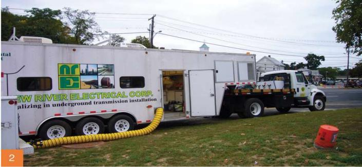
1. Underground cable comes on trucks specifically designed for the installation of underground cable. Crews will pull cable from one splice vault to another along the project route.
